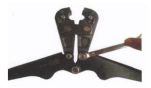
2. Loosen "LH" or "RH" back nuts with a spanner. Adjust the dial one increment at a time
