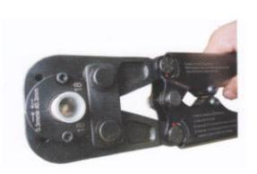
3. Stop the adjustment when the jaw interval <=0.3
